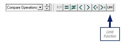
Insert a N/O contact and assign it to %S07, Always On. Next select the Limit function and insert it on the same Rung.
