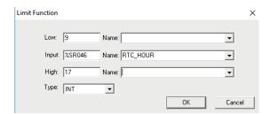
Insert the data shown to ensure that the hours are between 9am and 5pm. Finally enter a NO coil after the two Limit functions, assign it to %M01. This coil will be operated when both functions are true.
